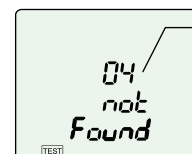
When incorrect wiring pattern cannot be detected
